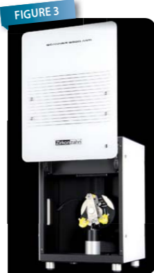
At the laboratory, the working casts were poured from the impressions, placed in the articulator and scanned using the fully automated, optical structured light scanner S600 ARTI. The software uses the articulator scan to determine the jaw relations and align the casts in perfect occlusion, allowing the identification and elimination of static and dynamic premature occlusal contacts.
