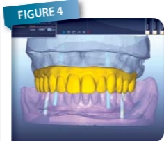
A digital waxup of the maxillary bridge was created using the Zirkonzahn.Modelier software and its "Heroes Collection" tooth set library (the software also offers a wizard with step-by-step design instructions). The customized titanium bases were modified on screen to optimize the orientation of the screw-access channels. The software then analyzed the digital waxup situation and adapted it to the gingival and implant geometries.
